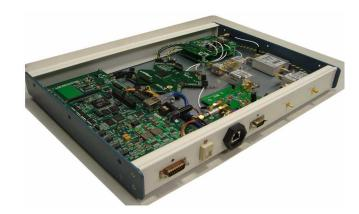
Fig. 9. The Cornell GRID receiver – the hardware platform for the receiver-spoofer.
