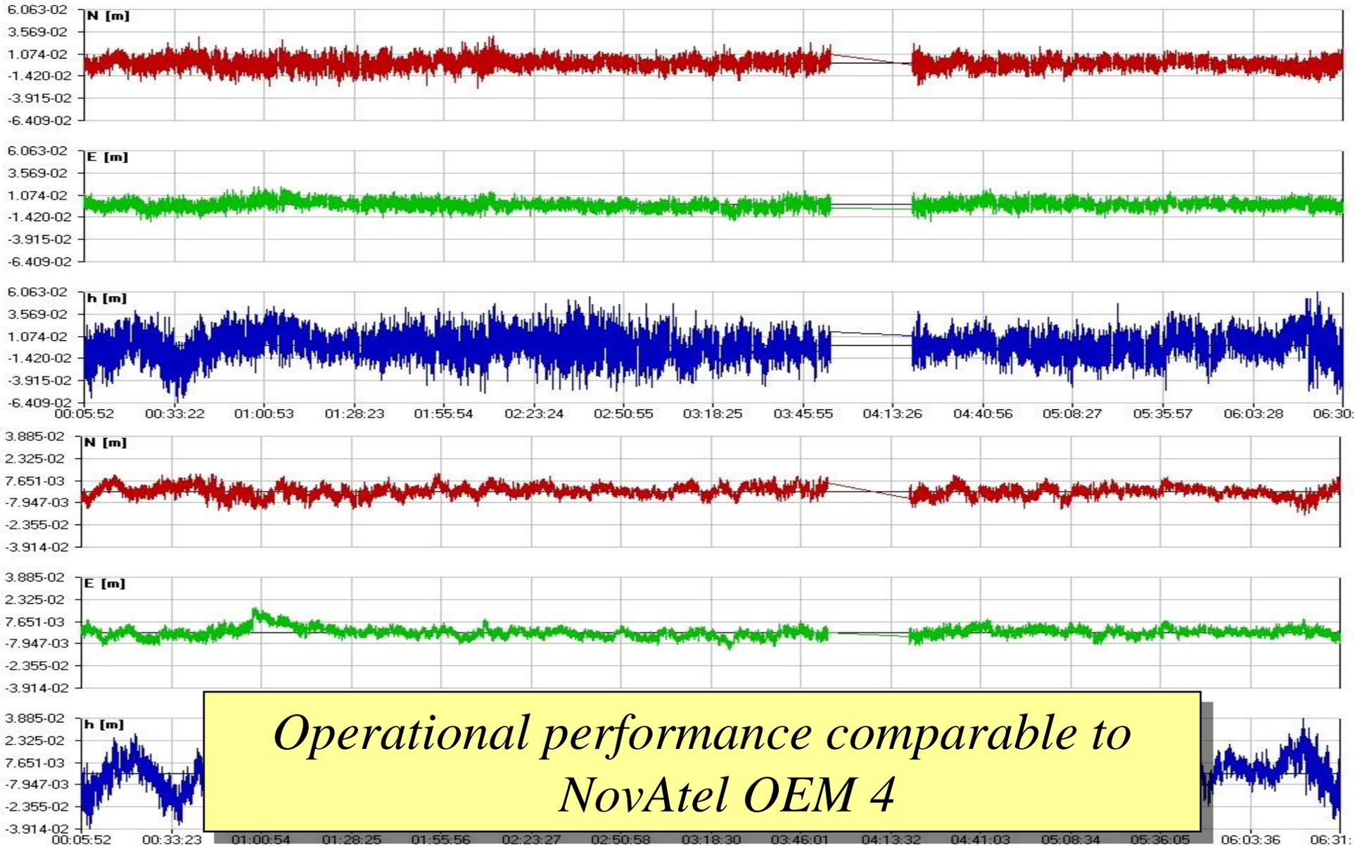
Coordinate time series of final PDGPS adjustment. Software receiver at top, OEM IV at bottom.
