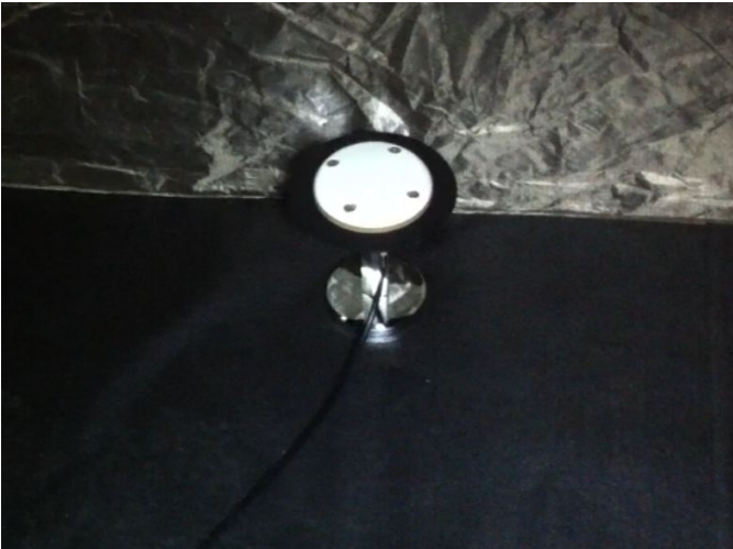
Fig. 5. The receive antenna inside the RF shielded tent which was receiving both the authentic and spoofed signals to feed to the target receiver.
