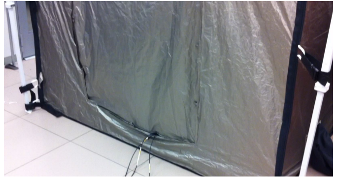
Fig. 3. RF shielded tent exterior with cables for the antennas.
