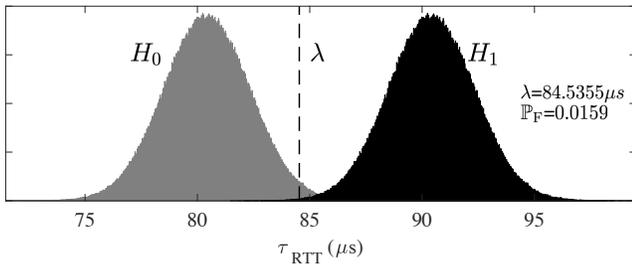
Fig. 8. Distribution of the test statistic under  $H_0$  and  $H_1$  for 80 RTT measurements per decision epoch. ( $N = 10$ ,  $\rho = 0.3$ ,  $L_M + \xi = 10\mu\text{s}$ ,  $\mathbb{P}_D = 0.999$ )
