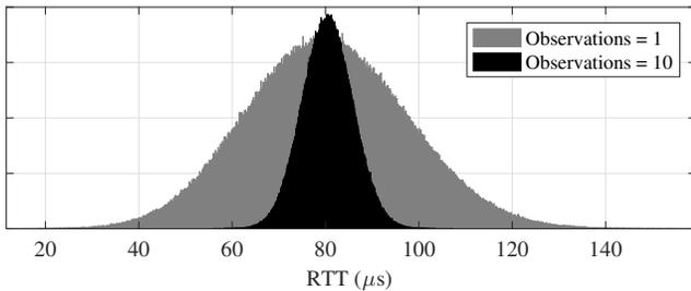
Fig. 6. Empirical distribution of the RTT of *sync-response* pairs through a network of  $N = 10$  routers with network idle probability of  $\rho = 0.3$ . The light-shaded histogram shows the empirical distribution of the RTT of a single *sync-response* pair. The dark-shaded histogram shows the corresponding distribution for the mean of batches of 10 observations of the RTT.
