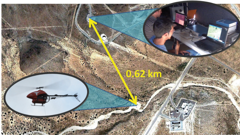
▲ FIGURE 2 Aerial view of the test site showing the spoofer location on a hilltop and the UAV site 0.62 kilometers away.
