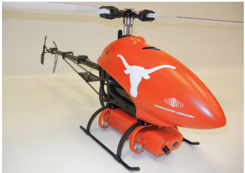
▲ UNMANNED AERIAL VEHICLE (UAV) used in the spoofing tests; owned by the University of Texas.
